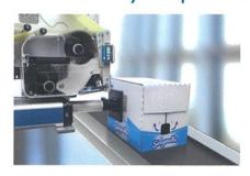
With the M230i-T4 and M230i-T6 you can choose the effective stroke length that is most suitable for your business. We offer three standard stroke lengths, I 60mm, 360mm and 560mm. Thanks to a very small footprint and a smart design it is possible to get close to the product, making installations easy on constrained production lines.
